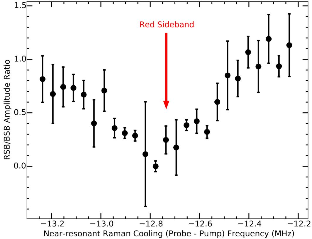
FIG. 8. Near-resonant Raman frequency scan around the RSB while measuring the RSB/BSB amplitude ratio (ion temperature) with 10 ms of sideband cooling. The minimum amplitude ratio is reached while sitting on the peak of the red sideband measured by the near-resonant Raman fluorescence. Data points were taken randomly and interleaved. Error bars are given by the propagation of the the least squares curve fit errors for the red and blue sideband amplitudes.
