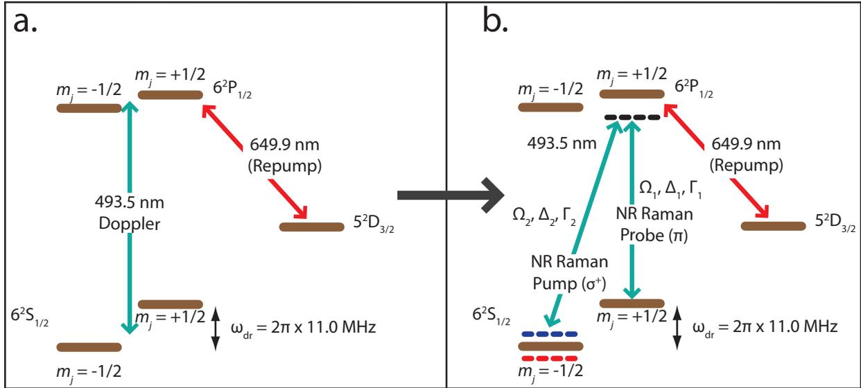
FIG. 3. Stages of  $^{138}\text{Ba}^+$  cooling. Solid lines show applied laser drives. Horizontal dashed lines show the red and blue motional sidebands of the driven Raman transition when relevant and the virtual state of the Raman transition (black), detuned by  $\approx 80$  MHz. (a) Doppler cooling lasts 20 ms. (b) Near-resonant Raman sideband cooling lasts either 1 or 10 ms. The PMT is gated with the near-resonant Raman beams.
