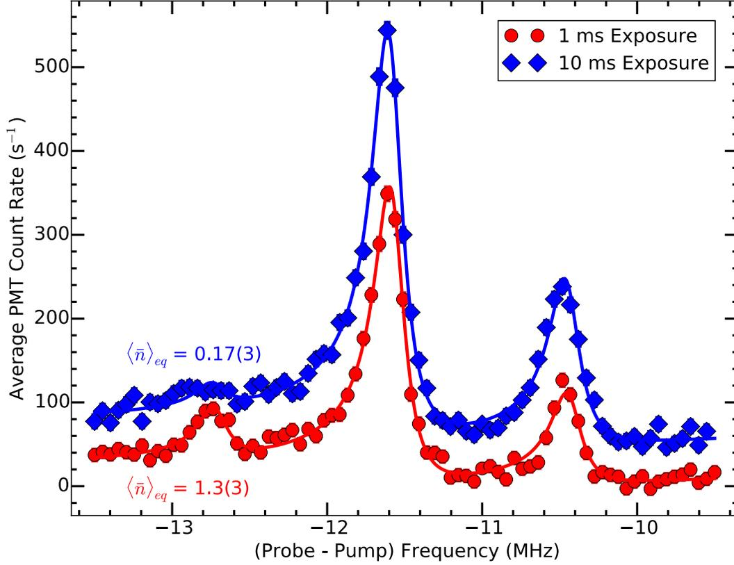
FIG. 4. Near-resonant Raman 493 nm fluorescence spectrum with red and blue motional sidebands resolved. The red circles (blue diamonds) are data corresponding to PMT exposure for the first 1 (10) ms of near-resonant Raman exposure. Solid lines are fits that can be used to extract equilibrium-equivalent occupation numbers,  $\langle \bar{n} \rangle_{eq}$ , discussed in Sec. III. Error bars are given by the standard deviation of the mean of each data point, and are comparable to the marker size.
