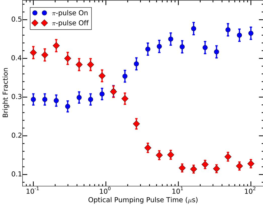
FIG. 9. Determination of optimal optical pumping time for the step shown in Fig. 5c. Far-off-resonant  $\pi$ -pulse off (red diamonds). Far-off-resonant  $\pi$ -pulse on (blue circles). We see that the minimum optical pumping time for minimum (maximum) bright fraction with the far-off-resonant  $\pi$ -pulse off (on) is  $\approx 10 \mu s$ . Data points in each data set were taken randomly and interleaved. Error bars are given by binomial statistics.
