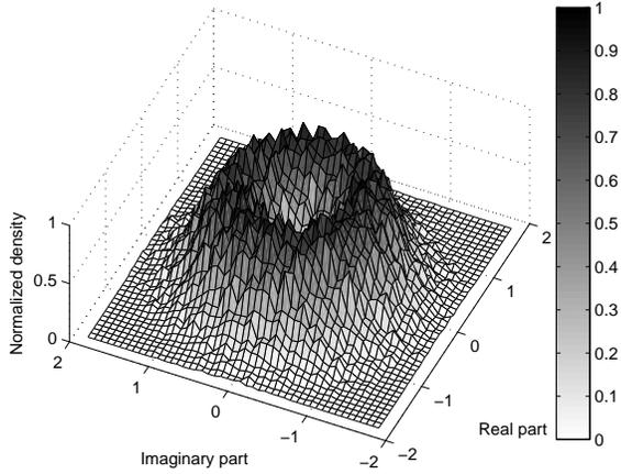
Fig 3. Histogram of elements of channel vector with  $r_{ijc} = 0.5$  (large angular spread or nearly NLOS)
