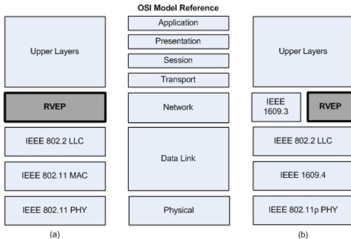
**Fig. 3.** RVEP in the network layers: (a) RVEP as a replacement of IP in nodes equipped with radios based on IEEE 802.11, and (b) RVEP as a replacement of IP in nodes equipped with radios based on IEEE 802.11p
