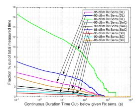
Fig. 3 Continuous outage duration below a given  $R_x$  sensitivity, with  $T_x$  power of 0 dBm, from agglomerate off-body data for direct link (DL), switchand-examine combining (SwC) and selection combining (SC)
