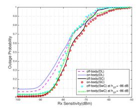
**Fig. 1** Outage probability as a function of receive sensitivity, with  $T_x$  power of 0 dBm, for direct link (DL), switch-and-examine combining (SwC) and selection combining (SC)
