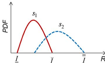
Fig. 2. An illustration of the information rates  $\underline{\underline{I}}$ ,  $\check{I}$  and  $\bar{\bar{I}}$  for a two-state channel. Solid and dashed lines indicate the asymptotic distributions of the information density rate  $n^{-1}i(X^n; Y^n|s)$  under the two states  $s_1$  and  $s_2$ .
