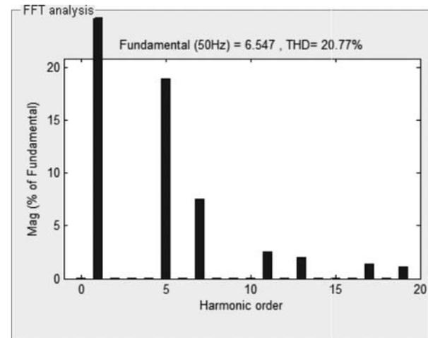
FIG. 5 SUPPLY CURRENT SPECTRUM BEFORE FILTERING
