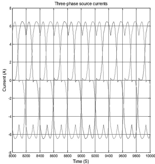
FIG. 4. SUPPLY CURRENTS WAVEFORMS BEFORE FILTERING
