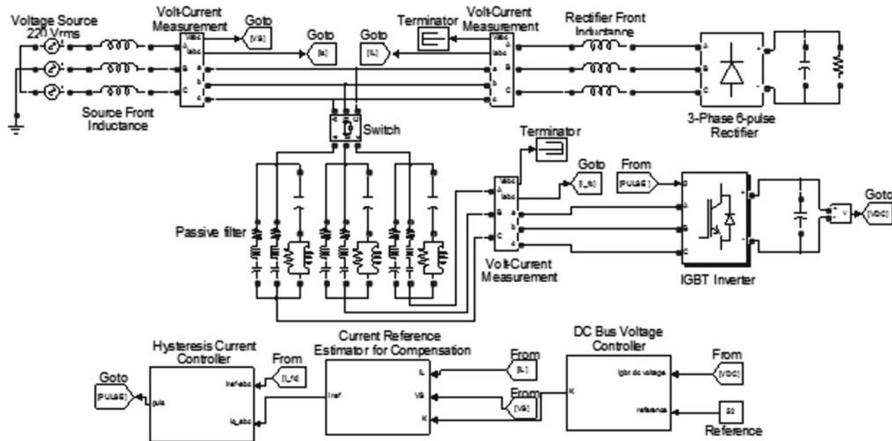
FIG. 1. GENERAL STRUCTURE OF HYBRID ACTIVE POWER FILTER AND ITS CONTROL
