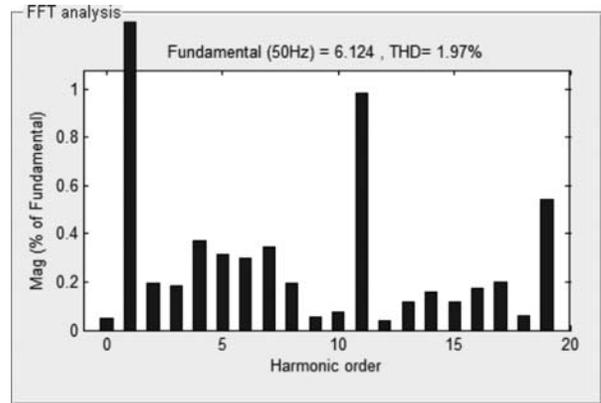
FIG. 8. SPECTRUM OF SOURCE CURRENT AFTER FILTERING
