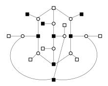
Fig. 10. An example of a subgraph in a  $(3, \rho, 8)$ -LDPC code which satisfies all conditions of Theorem 1 except the condition (b). This structure is not harmful for the PBF algorithm.
