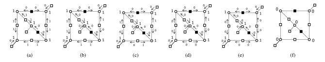
Fig. 16. The (5,3) trapping set in a column-weight three code that is eliminated if two super checks corresponding to a 2-error correcting component code are replaced. Arrows show messages from check nodes to variable nodes in each iteration of the Gallager B decoding algorithm: (a)-(d) messages from checks in iterations 1 to 4, (e) all variable nodes are corrected after the fourth iteration.
