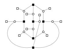
Fig. 9. A fixed set for a  $(3, \rho, 8)$ -LDPC code in which each variable node is connected to exactly two super checks.
