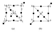
Fig. 2. The (5,3) trapping set is eliminated when all single parity checks are replaced by super checks corresponding to a 2-error correcting component code. (a) flip messages from super checks to corrupt variable nodes in the first iteration of the PBF algorithm, (b) all variable nodes are corrected after the first iteration.
