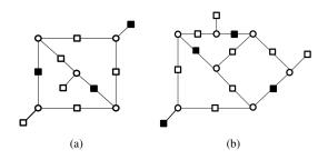
Fig. 11. Some trapping sets in a column-weight 3 LDPC codes that can be eliminated if each variable node is connected to exactly one super check. The graphs in (a) and (b) correspond to the (5,3) and (7,3) trapping sets, respectively.
