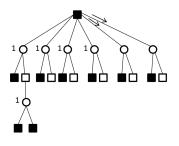
Fig. 18. A correctable error pattern of size 5 in which 4 corrupt variable nodes are connected to one super check and one error is connected to one single check.
