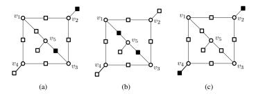
Fig. 4. Possible super-check replacements which are not helpful for the decoder to correct all errors on the (5,3) trapping set.
