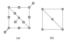
Fig. 7. (a) The (5,3) trapping set as a bipartite graph, (b) the simple graph induced by the 5 variable nodes of the (5,3) trapping set.
