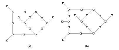
Fig. 8. (a) A (6,4) trapping set, (b) a (7,5) trapping set which is a subdivision of the (6,4) trapping set given in (a).
