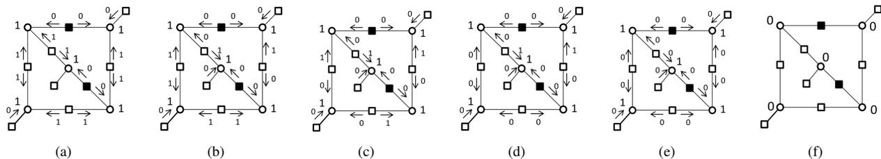
Fig. 16. The  $(5,3)$  trapping set in a column-weight three code that is eliminated if two super checks corresponding to a 2-error correcting component code are replaced. Arrows show messages from check nodes to variable nodes in each iteration of the Gallager B decoding algorithm: (a)-(d) messages from checks in iterations 1 to 4, (e) all variable nodes are corrected after the fourth iteration.
