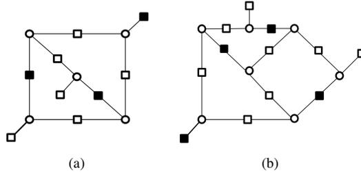
Fig. 11. Some trapping sets in a column-weight 3 LDPC codes that can be eliminated if each variable node is connected to exactly one super check. The graphs in (a) and (b) correspond to the  $(5,3)$  and  $(7,3)$  trapping sets, respectively.
