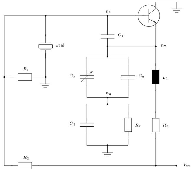
Fig. 2. Schematic of the 3MHz Colpitz-Quartz oscillator.
