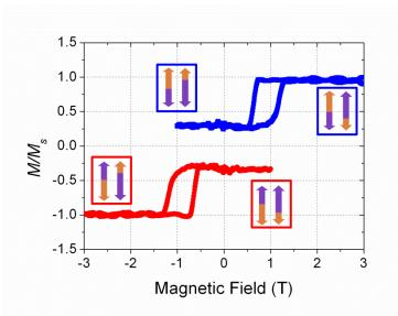
**Figure 2**. Experimental exchange bias minor loops of TbSmFeCo below  $T_{comp}$ . External field scans from 3 T through -1 T to 3 T (blue solid), and from -3 T through 1 T to -3 T (red solid). The arrows are defined similarly as **Figure 1**.
