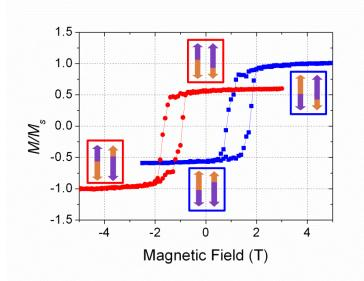
**Figure 5.** Simulated exchange bias minor loops of TbFeCo below  $T_{comp}$ . External field scans from 5 T through -3 T to 5 T (blue square), and from -5 T through 3T to -5 T (red circle). The arrows are defined similarly as **Figure 1**.
