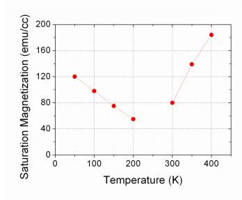
**Figure 3.** Temperature dependence of saturation magnetization simulated TbFeCo using the two-phase model.
