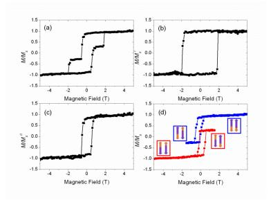
**Figure 4.** Simulated hysteresis loops of two-phase model. (a) Major loop of TbFeCo above  $T_{comp}$ , external field scans from 5 T to -5 T to 5 T. (b-c) Contribution to the major loop from Phase I (b) and Phase II (c) above  $T_{comp}$ . (d) Exchange bias minor loops of TbFeCo above  $T_{comp}$ . External field scans from 5 T to -1.1 T to 5 T (blue square), and from -5 T to 1.1 T to 5 T (red circle). The arrows are defined similarly as **Figure 1**.
