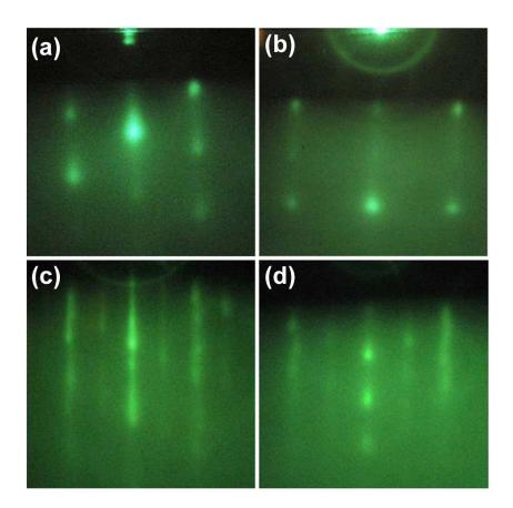
**Figure 3.** RHEED patterns for the bare MgO substrate with different incident electron beam azimuths taken form  $[1\overline{10}]$  and  $[11\overline{2}]$  direction (a), (b) before film growth and the corresponding patterns of the CuO thin film taken form [010] and [100] direction (c), (d) after film growth.
