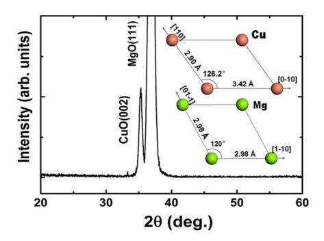
**Figure 1.** XRD spectrum of CuO(002) thin film grown on MgO(111) substrate. The inset is the sketch of Cu lattice in CuO(002) plane and Mg lattice in MgO(111) plane.
