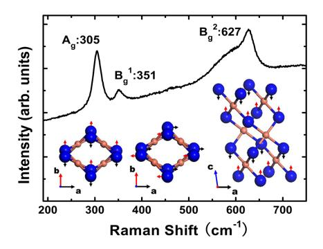
Figure 2. Raman spectrum of the CuO thin film and the corresponding O atoms vibration sketches of  $A_g$  mode,  $B_g^{-1}$  mode, and  $B_g^{-2}$  mode.
