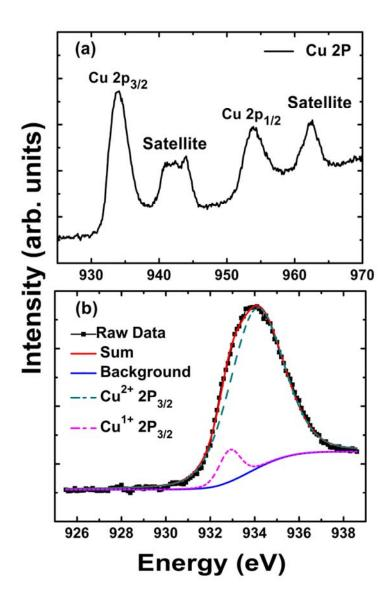
**Figure 4.** The raw data of Cu 2p XPS (a) and the fitting analysis of the Cu  $2p_{3/2}$  (b) spectra of the CuO thin film.
