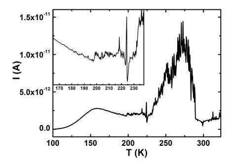
**Figure 5.** The temperature-dependent TSC of the CuO thin film along [010] direction, and the inset is the enlarged version from 170 K to 230 K.
