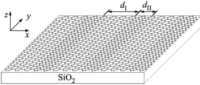
**Fig. 1.** Example of an array under study: graphene sheet on SiO<sub>2</sub> substrate with hydrogen atoms periodically deposited on graphene strips (graphene-graphane superlattice).
