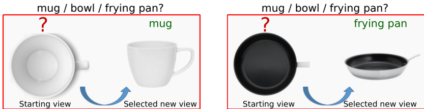
Fig. 1: A schematic illustrating the active categorization of two objects. A moving vision system may not recognize objects after just one view, but may intelligently choose to acquire new views to disambiguate amongst its competing hypotheses.
