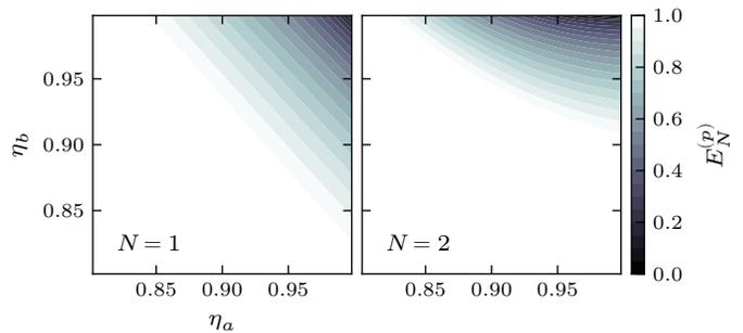
Figure 2: **Contour plot shows the effect of loss on the EPR steering:** EPR steering is observed when  $E_N^{(p)} < 1$ . The  $\eta_a$  and  $\eta_b$  are the efficiencies for detection of mode  $a$  and  $b$  respectively.
