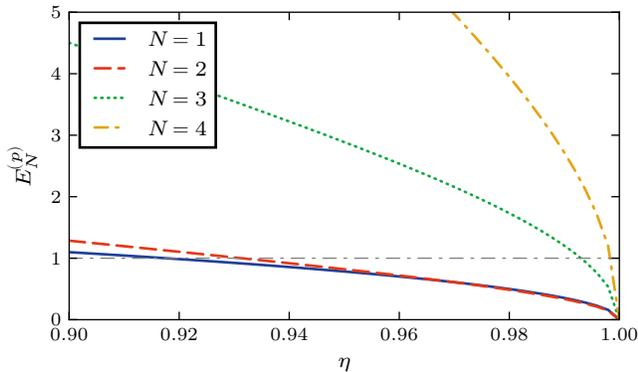
Figure 1: **Predictions for EPR steering of the NOON states.** EPR steering is observed when  $E_N^{(p)} < 1$ . It is assumed that the two-mode NOON state is created and that each mode is then (independently) subjected to losses. Loss at each mode is modeled by a beam splitter coupling as described in Sec. VI. Here the beam splitter transmission efficiencies are  $\eta = \eta_a = \eta_b$ . We select the NOON state (1) with  $\phi = 0$  for  $N$  odd and  $\phi = \pi/2$  for  $N$  even.
