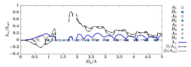
Figure 13: (Color online) Eigenvalues of the effective stiffness matrix  $\mathbf{L}_{\text{eff}}$  (see Eqs. (72) and (75)),  $\Lambda_{\alpha}/L_{\text{scl}}$ , as a function of the size parameter for the LG<sub>01</sub> beam with f = 0.3.
