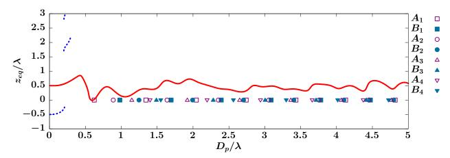
Figure 10: (Color online) On-axis coordinate of axially stable zero-force points  $z_{eq}$  as a function of the size parameter for the LG<sub>10</sub> beam.
