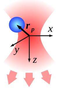
Figure 1: (Color online) Mie scatterer (spherical particle) is illuminated with a focused LG beam propagating along the z axis. The displacement vector  $\mathbf{r}_p$  determines location of the particle with respect to the beam waist.
