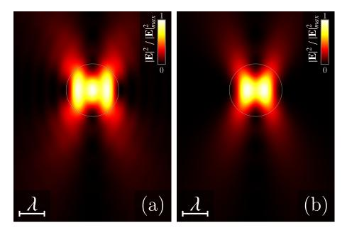
Figure 11: (Color online) Intensity distributions of the incident wave field in (a) the x - z plane and (b) the y - z plane for the LG<sub>01</sub> beam with f = 0.3. The z axis is directed from the top down.
