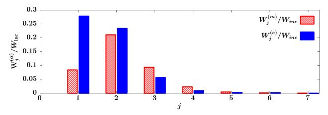
Figure 12: (Color online) Histogram of multipolar decomposition of the incident  $LG_{01}$  beam with f = 0.3. Height of the bars represents relative contribution of the modes,  $W_j^{(m)}/W_{inc}$  and  $W_j^{(e)}/W_{inc}$ , (see Eqs. (36) and (37)) to the total power of the incident beam depending on the angular momentum number j.
