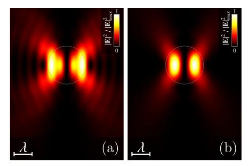
Figure 15: (Color online) Intensity distributions of the incident wave field in (a) the x - z plane and (b) the y - z plane for the LG<sub>02</sub> beam with f = 0.3. The z axis is directed from the top down.
