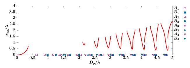
Figure 5: (Color online) On-axis coordinate of axially stable zero-force points  $z_{eq}$  as a function of the size parameter for the Gaussian beam.
