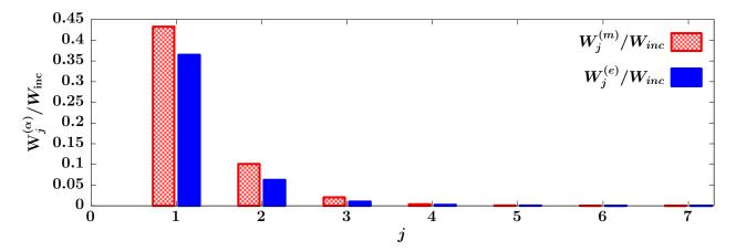
Figure 3: (Color online) Histogram of multipolar decomposition of the incident  $LG_{00}$  (Gaussian) beam with f = 0.3. Height of the bars represents relative contribution of the modes,  $W_j^{(m)}/W_{inc}$  and  $W_j^{(e)}/W_{inc}$ , (see Eqs. (36) and (37)) to the total power of the incident beam depending on the angular momentum number j.
