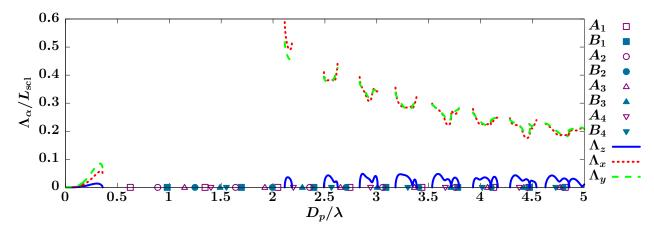
Figure 4: (Color online) Eigenvalues of the effective stiffness matrix  $\mathbf{L}_{\text{eff}}$  (see Eqs. (72) and (73)),  $\Lambda_{\alpha}/L_{\text{scl}}$ , as a function of the size parameter,  $D_p/\lambda = 2R_p/\lambda$ , for the LG<sub>00</sub> beam with f = 0.3. The scale factor is  $L_{\text{scl}} = nW_{\text{inc}}/(c\lambda m_p)$  (see Eq. (72)) and the refractive index of the particle is  $n_p = 1.33$ .
