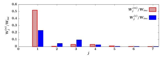
Figure 8: (Color online) Histogram of multipolar decomposition of the incident LG<sub>10</sub> beam with f = 0.3. Height of the bars represents relative contribution of the modes,  $W_j^{(m)}/W_{\text{inc}}$ and  $W_j^{(e)}/W_{\text{inc}}$ , (see Eqs. (36) and (37)) to the total power of the incident beam depending on the angular momentum number j.
