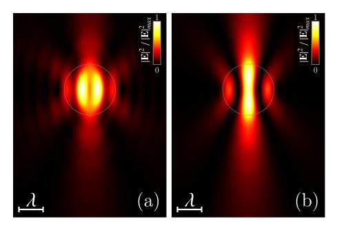
Figure 7: (Color online) Intensity distributions of the incident wave field in (a) the x - z plane and (b) the y - z plane for the non-vertex LG<sub>10</sub> beam with f = 0.3. The z axis is directed from the top down.
