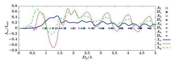
Figure 9: (Color online) Eigenvalues of the effective stiffness matrix  $\mathbf{L}_{\text{eff}}$  (see Eqs. (72) and (73)),  $\Lambda_{\alpha}/L_{\text{scl}}$ , as a function of the size parameter for the LG<sub>10</sub> beam with f = 0.3. The scale factor is  $L_{\text{scl}} = nW_{\text{inc}}/(c\lambda m_p)$  (see Eq. (72)).
