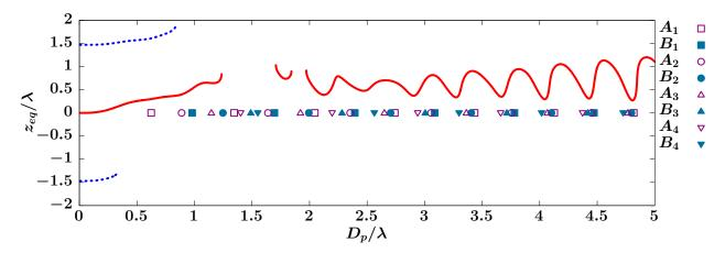
Figure 14: (Color online) On-axis coordinate of axially stable zero-force points  $z_{eq}$  as a function of the size parameter for the LG<sub>01</sub> beam.
