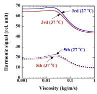
**Figure 8:** Simulation results of the relationship between the 3rd (solid lines) or 5th harmonic signal (dashed lines) and viscosity for temperatures of 27 °C and 37 °C. In these cases, SPIONs were assumed to consist of magnetite (Fe<sub>3</sub>O<sub>4</sub>), and  $\sigma$  in equation (15) and E(D) in equation (16) were taken as 0.282 and 17.1 nm, respectively. The peak-to-peak strength and frequency of AMF were assumed to be 20 mT and 400 Hz, respectively.
