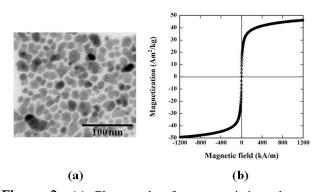
**Figure 2:** (a) Photograph of a transmission electron microscope (TEM) image of the SPIONs used in this study (M-300). The calibration bar (100 nm) is also shown. (b) Magnetization curve of M-300 as a function of magnetic field, which was measured using a vibrating sample magnetometer.
