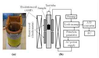
**Figure 1:** Photograph (a) and diagram (b) of our apparatus for measuring blood coagulation. The alternating magnetic field (AMF) was generated using an excitation (solenoid) coil whose AC power was supplied by a programmable power supply. The signals generated by superparamagnetic iron oxide nanoparticles (SPIONs) were received by a gradiometer coil, and the 3rd and 5th harmonic signals were extracted using a preamplifier and a lock-in amplifier.
