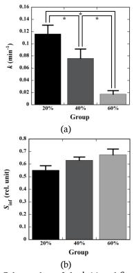
**Figure 6:** Column plots of the k (a) and  $S_{inf}$  values (b) calculated by fitting the time course of the normalized 3rd harmonic signal (figure 5(a)) to equation (1) for groups with hematocrits of 20%, 40%, and 60%. \* P<0.05.
