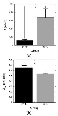
**Figure 4:** Column plots of the coagulation rate (k) (a) and the normalized signal intensity at infinite time  $(S_{inf})$  (b) calculated by fitting the time course of the normalized 3rd harmonic signal (figure 3(a)) to equation (1) for groups with CaCl<sub>2</sub> solution added and kept at room temperature (27 °C) and 37 °C. \* P<0.05.
