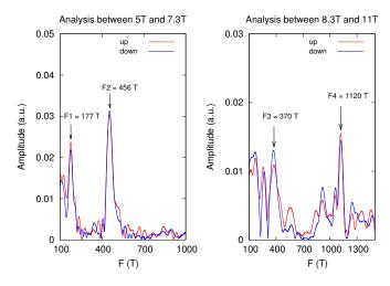
FIG. 6. Fourier analysis of the data shown in Fig. 5. The main frequencies are the  $456\,\mathrm{T}$  in the low-field region and  $1120\,\mathrm{T}$  in the high-field region.
