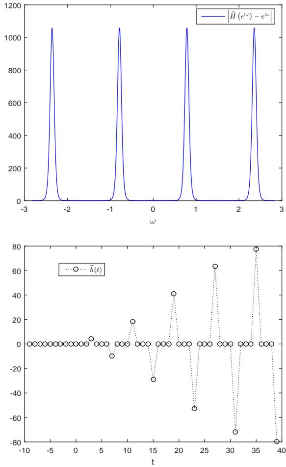
Figure 1: Approximation of the one-step forward shift operator: the values  $|\hat{H}(e^{i\omega}) - e^{i\omega}|$  for the transfer function of the predictor (4) and the values of the corresponding kernel  $\hat{h} = \mathcal{Z}^{-1}\hat{H}$  with  $\gamma = 4$ ,  $r = 0.4$ ,  $m = 4$ .
