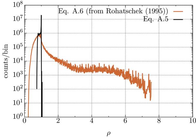
Figure A.6: Parameter sweep histogram for  $63 \cdot 10^6$  parameter combinations. The parameter sweep intervals are given in Tab. 2.  $\rho$  (Eq. 36) is the ratio of the corresponding approximation of the photophoretic force and the total of the effectively exact numerical result given by Eq. 7, where the surface temperatures were numerically obtained with COMSOL. The bin size is 0.005 (0.5%).
