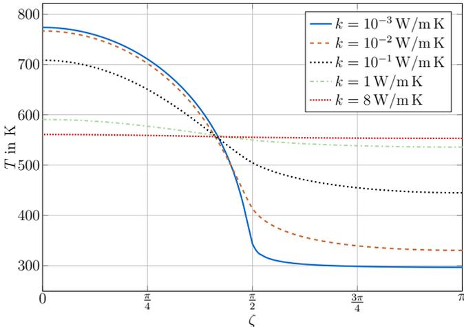
Figure 2: Temperature distribution across the surface of a sphere with  $r_0 = 0.66$  mm at different thermal conductivities, along the model setup shown in Fig. 1. The intensity is  $I_0 = 20 \text{ kW m}^{-2}$  ( $\varepsilon = 1$ ), the radiation temperature is  $T_{\text{rad}} = 293 \text{ K}$  at  $h = 0 \text{ kW m}^{-2} \text{ K}^{-1}$ .
