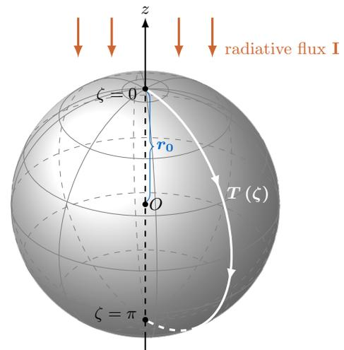
Figure 1: Visualization of the situation considered. Illumination is directed along  $z$ -axis, thus for a homogeneous particle the surface temperature only depends on  $\zeta$  (spherical coordinate system  $(r, \xi, \zeta)$ ). The sphere's radius is  $r_0$ . Gas particles impinge at temperature  $T_g^\ominus$  and scatter at  $T_g^\oplus$ .
