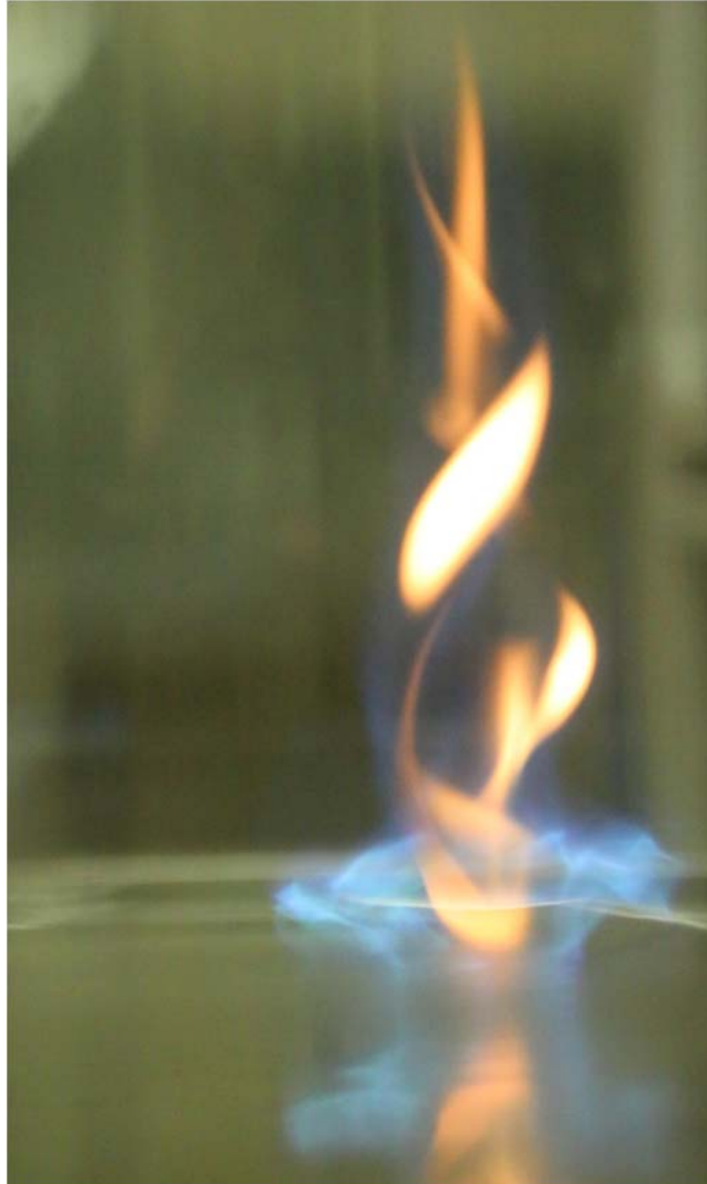
Figure 3. Transitioning whirl during the evolution process from a yellow fire whirl to a blue whirl. The height of this structure is about 15 cm. A cup-like blue whirling flame on water holds a yellow whirling flame.
