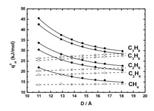
Figure 8. Zero-coverage isosteric heats of adsorption on the bundle's interior (filled symbols) and exterior volume (open symbols). Calculated values at 18.1 Å for  $CH_4$ ,  $C_2H_6$  and  $C_2H_4$  do not consider interstitial confinement (see text for details). Symbols are calculated data and lines are either linear (dashed) or first order exponential (solid) decays (eqn. 5).
