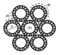
Figure 1. Different adsorption sites on an homogeneous bundle of SWCNTs with individual tube diameter D: (1) intratubular, (2) interstitial channel, (3) external groove, (4) external rounded surface. Sites 1 and 2 comprise the internal pore volume of the bundle, whereas sites 3 and 4 are both located on the exposed surface of the outermost nanotubes.
