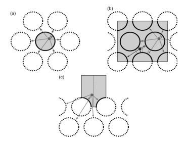
Figure 2. Cross sections of the unit simulation boxes for GCMC simulation of fluid adsorption onto different adsorption sites of an homogeneous bundle of open-ended SWNTs: *a*) intratubular volume; *b*)
