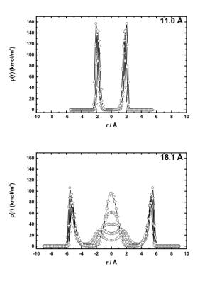
Figure 6. Radial concentration profiles on the intratubular volume of a bundle at  $(p / p_0) = 0.9$ . Results for  $C_2H_4$  and  $C_3H_6$  at 11.0 Å are not plotted for simplicity sake, although the results are analogous to  $C_2H_6$  and  $C_3H_8$  (see text for details). O  $CH_4$ ,  $\Delta C_2H_6$ ,  $\nabla C_2H_4$ ,  $\Delta C_3H_8$ ,  $\Delta C_3H_6$ .
