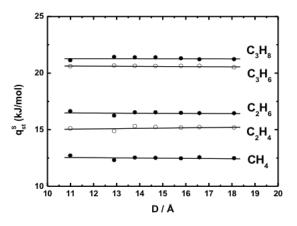
**Figure 7.** Isosteric heats of adsorption on the bundle's external rounded surface as function of individual tube diameter. Note the constancy of all calculated data, whose average errors are smaller than the symbols size.
