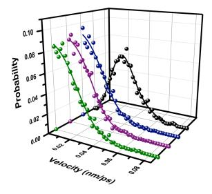
Figure 6. Velocity probability profiles of confined dsDNA. Instant velocities were calculated for the entire observation time window (80 ns) and histogram reweighted with a bin width of 0.002 nm/ps: *black*) molecular center of mass (3D), *blue*) z-component, *green*) x-component and *purple*) y-component. Symbols correspond to histogram data and lines are the best statistical fittings (*cf.* Section 2.3); analysis along any individual direction (x, y, z) includes only the decay region.
