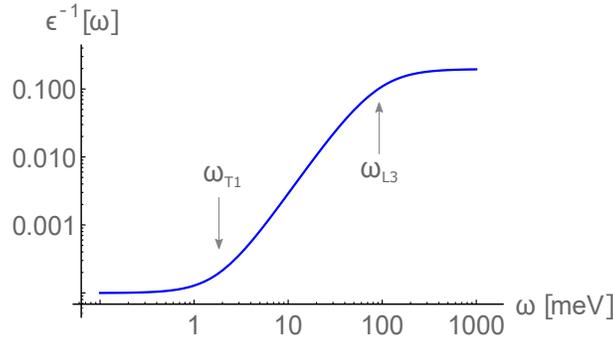
FIG. 5. The dielectric function Eq. 9 in insulating SrTiO<sub>3</sub> as a function of Matsubara frequency.
