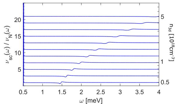
FIG. 4. The superconducting TDOS  $\nu_{sc}(\omega)$  divided by the normal TDOS  $\nu_N(\omega)$  for different values of the density calculated from the analytic continuation of Eq. 6. The curves are shifted from each other by 2 to make them distinguishable. The resonant feature appearing around  $\omega = \omega_0$  depends strongly on the electronic density and is therefore a 'finger print' of plasmonic superconductivity. The gap is barely observable on this scale.
