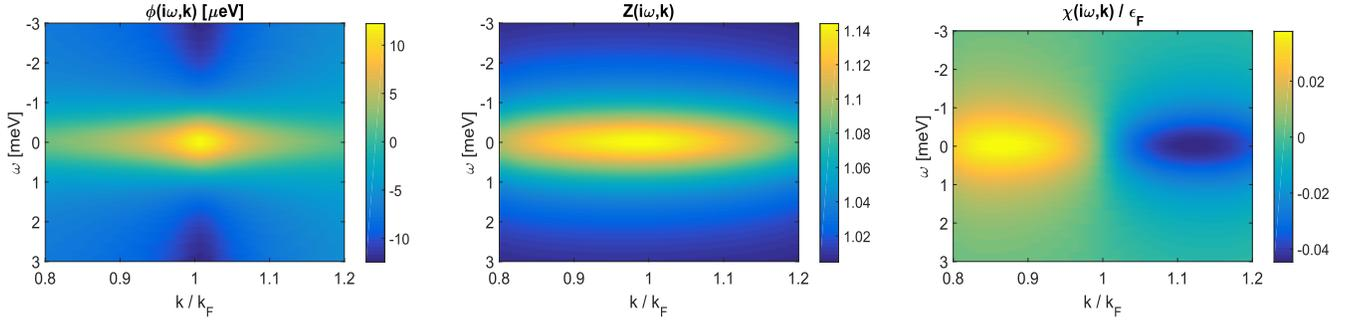
FIG. 11. The numerical solutions of the Eliashberg equations Eqs. 5 restricted to the vicinity of  $k = k_F$  for typical parameters used in this paper:  $n = 5 \times 10^{17} \text{ cm}^{-3}$ ,  $m = 2m_e$ ,  $\epsilon_F = 1.2 \text{ eV}$ ,  $\omega_- = 2\epsilon_F/3$ ,  $\eta = 0.4$ ,  $\alpha = 5 \times 10^{-16} \text{ cm}^3$  and  $T = 20 \text{ mK}$ .
