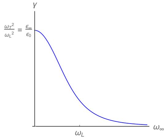
FIG. 7. The coupling constant  $\gamma$  as a function of the bare plasma frequency. Once the plasma frequency becomes larger than the longitudinal phonon frequency  $\omega_L$  it completely shields it and the coupling goes to zero.
