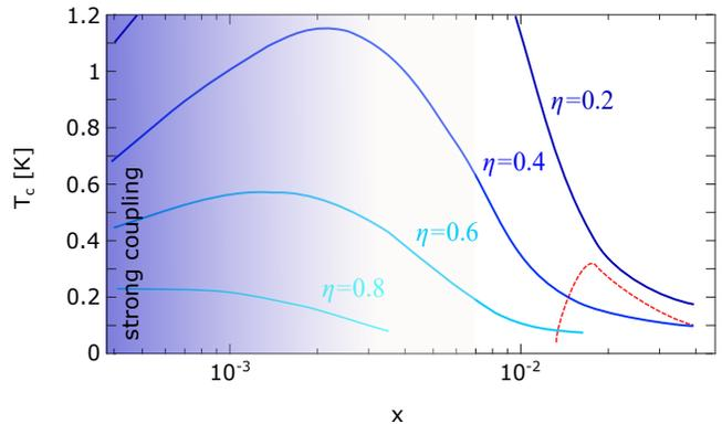
FIG. 3. The transition temperature in two-dimensions vs. doping for  $\omega_T = 15 \text{meV}$  and  $m = m_e$  and for  $\eta = 0.2, 0.4, 0.6$  and  $0.8$ . The red dashed line is the typical  $T_c$  from experiments [36]. The region of strong coupling where the calculation is not valid is shaded.
