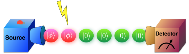
FIG. 1: The quantum change point problem. A quantum source emits particles in a default state |0\rangle , until the point where a mutation occurs, causing the source to emit particles in a different state |\phi\rangle . A detector receives the stream of particles emitted from the source and measures them, producing an estimate of the point where the mutation occurred.
