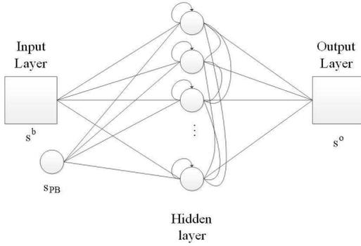
Figure 2: Recurrent Neural Network with Parametric Bias Units
