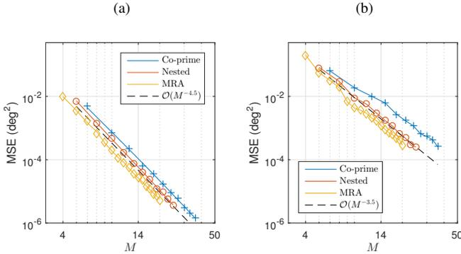
Fig. 6. MSE vs.  $M$ : (a)  $K = 1$ , (b)  $K = M$ . The solid lines are analytical results. The “+”, “o”, and “ $\diamond$ ” denote empirical results obtained from 500 trials. The dashed lines are trend lines used for comparison.
