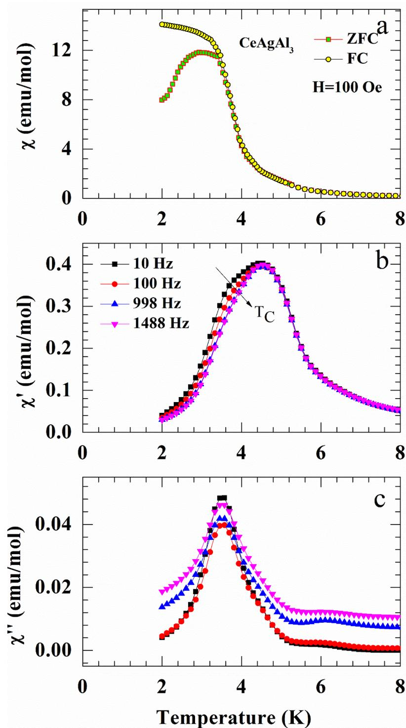
**Fig.3.** dc and ac magnetic susceptibility of CeAgAl<sub>3</sub>. (a). dc magnetic susceptibility measured under ZFC and FC conditions. (b). Real part  $\chi'$  and (c) Imaginary part  $\chi''$  of ac susceptibility measured at various frequencies such as 10, 100, 998, 1488 Hz for  $H_{ac} = 2.5$  Oe.
