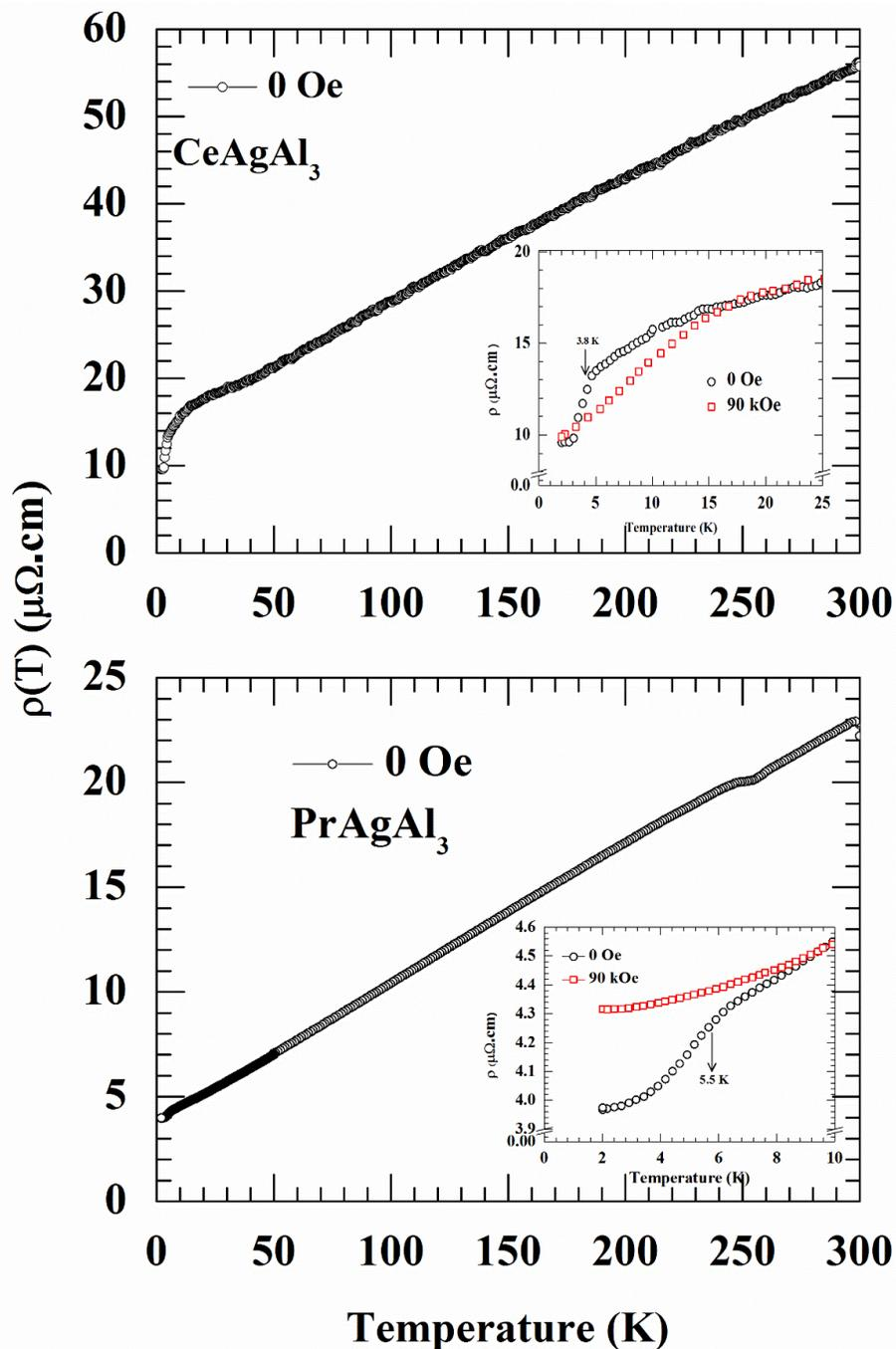
**Fig. 9.** Electrical resistivity  $\rho(T)$  of  $\text{RAgAl}_3$  ( $\text{R} = \text{Ce}$  and  $\text{Pr}$ ) measured in zero and 90 kOe field. Insets show the low temperature  $\rho(T)$  versus temperature.
