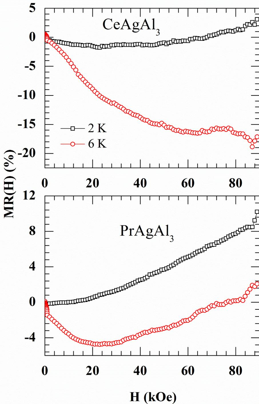
**Fig.10.** Magnetoresistance of  $\text{RAgAl}_3$  ( $\text{R} = \text{Ce}$  and  $\text{Pr}$ ) at 2 K and 6 K as function of magnetic fields up to 90 kOe
