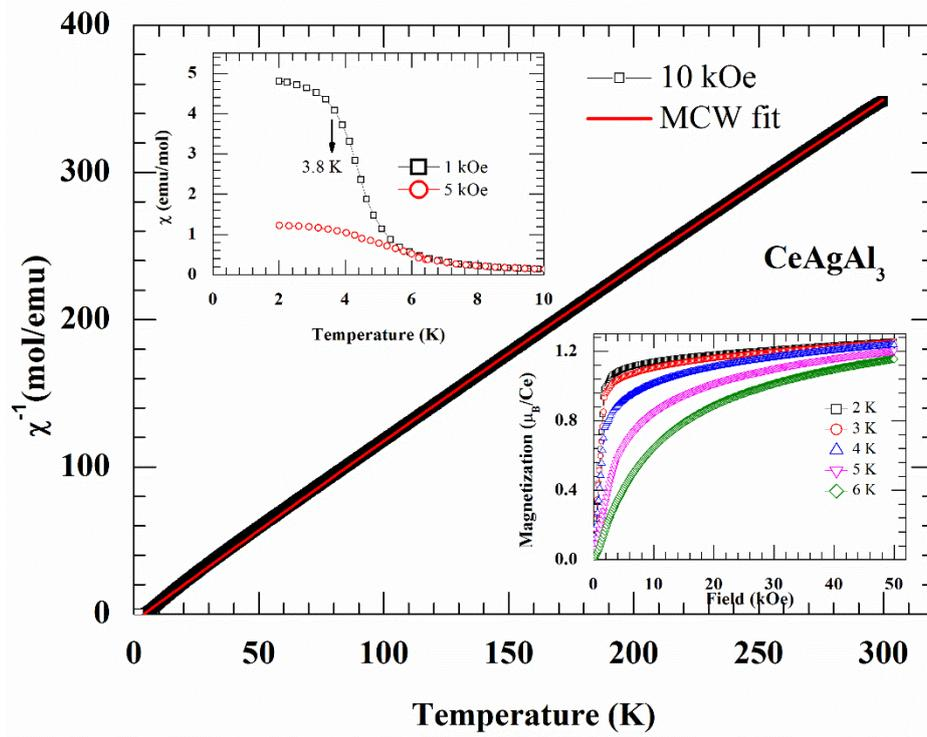
**Fig.2.** Inverse magnetic susceptibility of CeAgAl<sub>3</sub>. The upper inset shows susceptibility ( $\chi$ ) in 1 and 5 kOe below 10 K. The lower inset shows isothermal magnetization versus applied field at selected temperatures.
