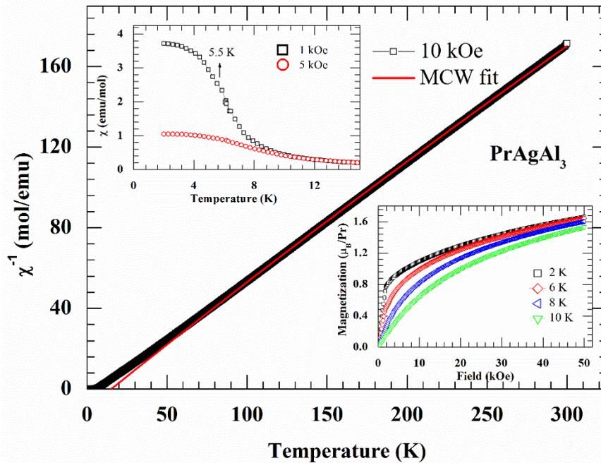
**Fig. 4.** Inverse magnetic susceptibility of  $\text{PrAgAl}_3$ . The upper inset shows susceptibility ( $\chi$ ) in 1 and 5 kOe below 15 K. The lower inset shows isothermal magnetization versus applied field for different temperatures.
