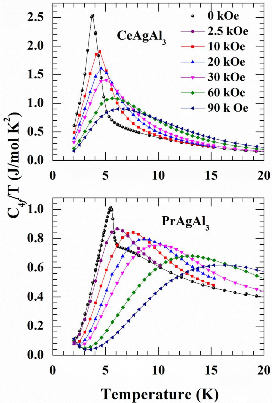
**Fig. 8.** The plots of  $C_{4f}(T)/T$  versus  $T$  for  $\text{RAgAl}_3$  ( $R = \text{Ce}$  and  $\text{Pr}$ ) in various applied magnetic fields.
