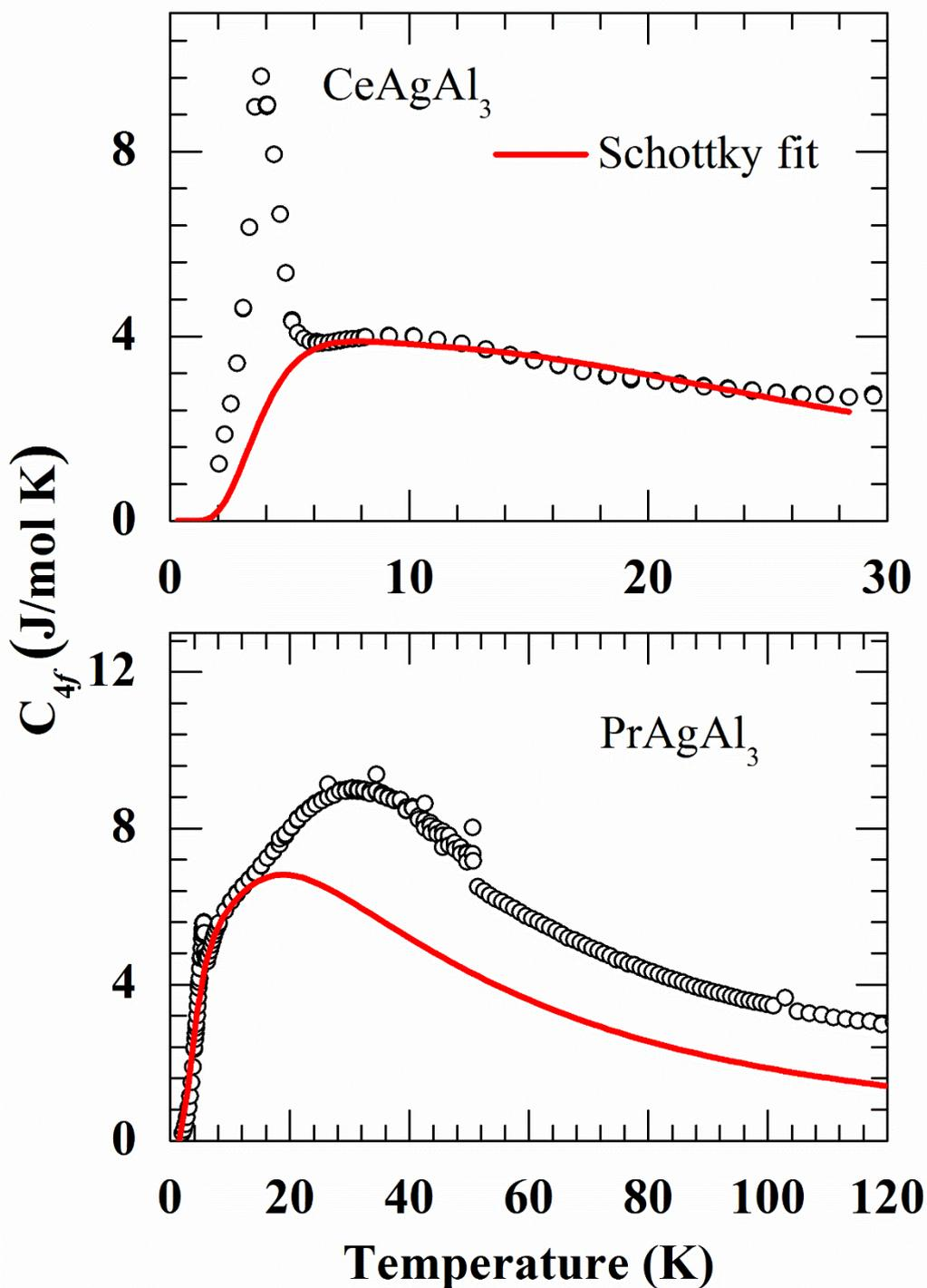
**Fig.6.** Temperature dependence of the 4f-derived specific heat ( $C_{4f}$ ). In both figures, the solid lines represent the fits to the expression of Schottky heat capacity equation (3).
