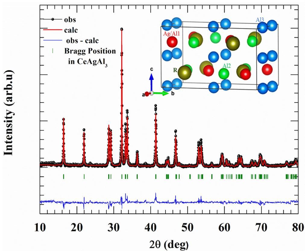
**Fig.1.** Powder X-ray diffraction pattern of orthorhombic CeAgAl<sub>3</sub> along with Rietveld refinement using GSAS program. The inset shows the crystal structure of RAgAl<sub>3</sub> (R = La, Ce and Pr). The atoms are represented by different colours and ball size. The dark line shows the unit cell.
