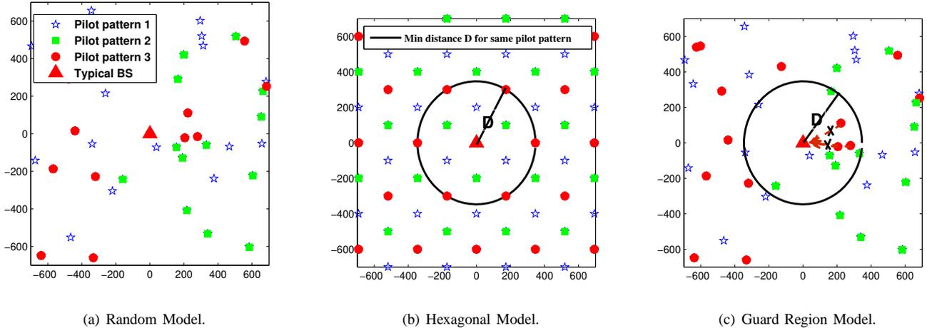
Fig. 1. Illustration of one realization of BS position from guard region PPP model, compared to random PPP model and ideal hexagonal model, with the same BS density ( $\lambda_B = 2.8 \times 10^{-5}$  [BSs per  $m^2$ ]),  $K = 10$  per cell and pilot reuse factor  $\Delta = 3$ .
