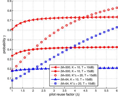
Fig. 4. Relation between pilot reuse factor  $\Delta$  and SINR requirement  $\gamma$  in (8), with  $\sigma^2 = 0$ ,  $\varepsilon = 0.5$  for  $T \in \{10 \text{ dB}, 15 \text{ dB}\}$  and  $M \in \{64, 500\}$ .
