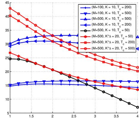
Fig. 5. Average cell throughput with respect to different pilot reuse factor  $\Delta$ , with  $\sigma^2 = 0$ ,  $T_{max} = 21 \text{ dB}$ ,  $\varepsilon = 0.5$  for  $T_C \in \{50, 200, 500\}$  and  $M \in \{100, 500\}$ .
