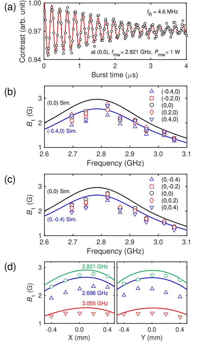
FIG. 5. (Color online) (a) An example of Rabi oscillations. The solid line is the fit. (b, c) Plots of  $B_1$  at  $P_{mw} = 1$  W for five positions along the X (b) and Y (c) axes. The solid lines are simulation results at (0, 0), (-0.4, 0) and (-0.4, 0) as indicated. (d) Experimental and simulated (solid lines) spatial distributions of  $B_1$  along the X (left) and Y (right) axes at three frequencies.
