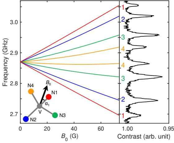
FIG. 4. (Color online) CW ODMR spectrum taken at the hole center (0, 0) (right) and calculated  $B_0$ -dependence of the transition frequencies at  $\alpha_1 = 29^\circ$ ,  $\alpha_2 = 132^\circ$ ,  $\alpha_3 = 109^\circ$ , and  $\alpha_4 = 83^\circ$  (left). At  $B_0 = 74$  G, the eight resonances are reproduced simultaneously.
