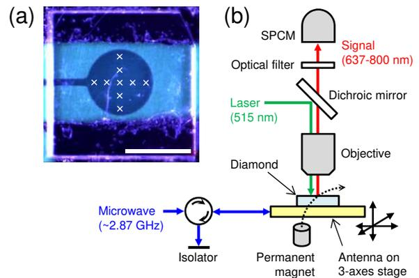
FIG. 3. (Color online) (a) An optical microscope image of the diamond sample mounted on the antenna. The scale bar is 1 mm. The cross marks (x) indicate the positions where ODMR measurements in Section IV are conducted. Their XY coordinates (in millimeter) are  $(0, 0)$ ,  $(0, \pm 0.2)$ ,  $(0, \pm 0.4)$ ,  $(\pm 0.2, 0)$ , and  $(\pm 0.4, 0)$ . (b) Schematic of experimental setup. SPCM: single photon counting module.
