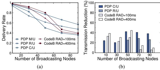
Figure 1: Performance under varying traffic load: (a) Delivery rate (b) Transmission reduction compared to PDP M/U.
