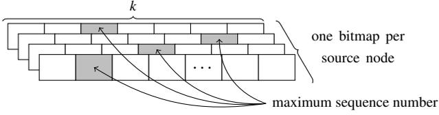
Figure 5: Structure used for the modified covered/uncovered (MC/U) termination criterion.
