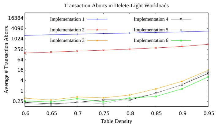
Figure 5: The average number of transaction aborts over the lifetime of tables filled to varying densities, for various transactional cuckoo hashing implementations, using a delete-light workload and 15 threads.
