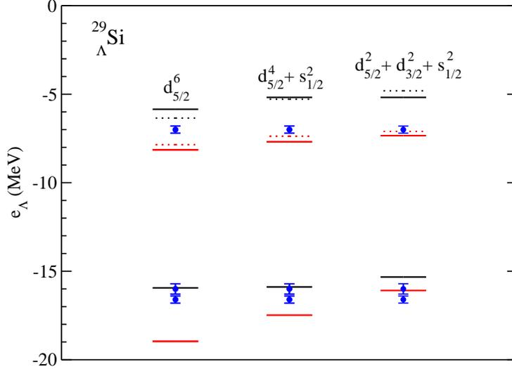
Figure 4: The  $\Lambda$  single particle energies in  $^{29}_{\Lambda}\text{Si}$  with three different configurations of the nuclear core, calculated within the mean-field model with realistic interactions (black lines) and the RMF model NL-SH (red lines). The  $0p_{1/2}$  levels are denoted by dotted lines. The energies of the  $s$  and  $p$  levels measured for  $^{28}_{\Lambda}\text{Si}$  are taken from [42, 43].
