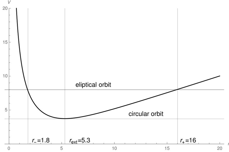
Fig. 2. Plot of  $V_{eff}(r)$ , with  $L = 14$ ,  $Q = 0$ .  $r_+ = a$ ,  $r_- = b$  are the turning-points corresponding to the maximum and minimum distance from the origin. For  $E = E_m$  the orbit degenerates into a circular orbit.
