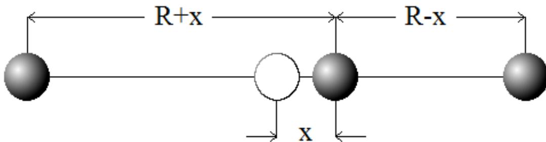
**Fig.7.** Simple model of 3 atoms interacting via Lennard-Jones potential. Atoms 1, 3 are fixed, while atom 2 is displaced by  $x$  from its old equilibrium position in origin.
