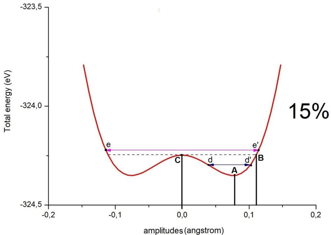
**Fig.5.** Carbyne potential plot for 15% strain and  $\pi$ -mode oscillations of carbon atom with respect to new (point A) and old (point C) equilibrium positions.
