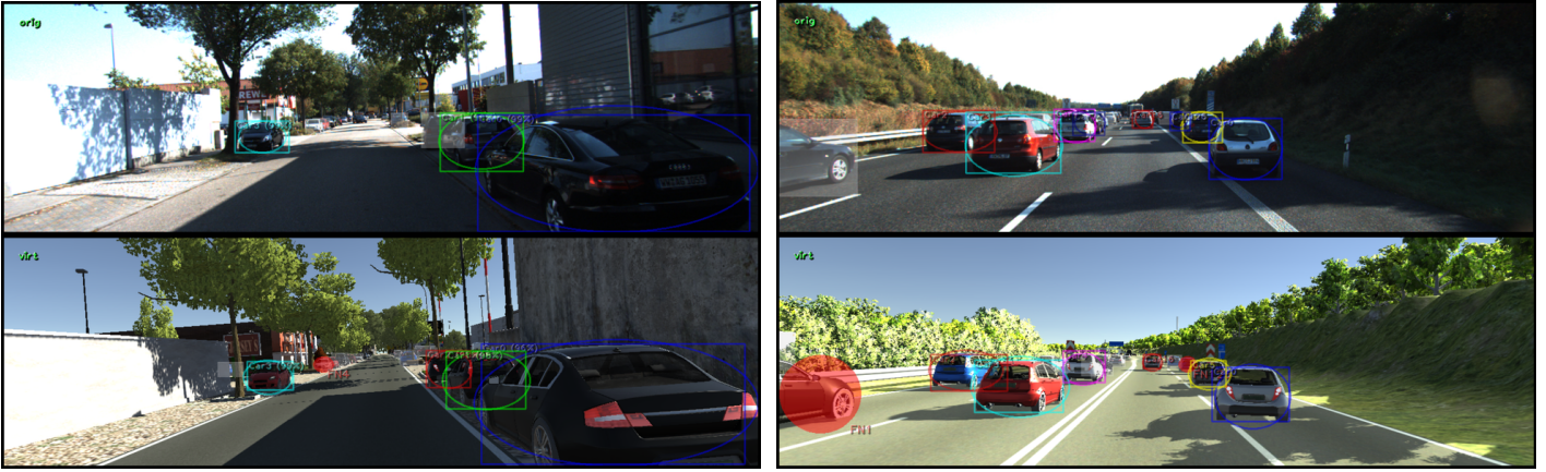
Figure 5: Predicted tracks on matching frames of two original videos (top) and their synthetic clones (bottom) for both DP-MCF (left) and MDP (right). Note the visual similarity of both the scenes and the tracks. Most differences are on occluded, small, or truncated objects.
