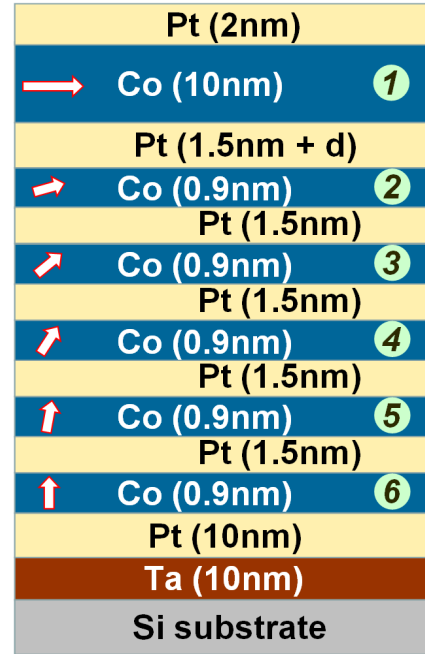
FIG. 1. (Color online) A schematic drawing of CoPt/Pt( d )/Co multilayer structure. Numbers of layers are shown on the right side; arrows on the left side demonstrate magnetization distribution.
