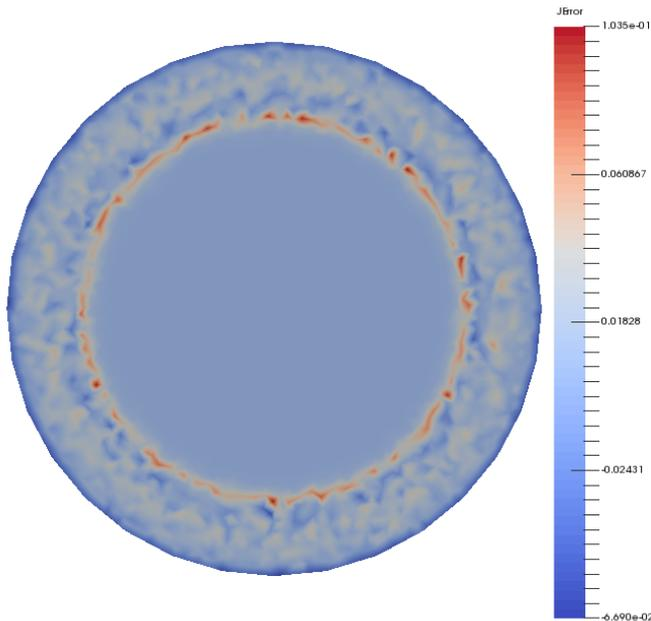
FIG. 8. Local  $L^2$  error of  $\nabla \times \mathbf{u}$  at  $t = 0.272$ . The scale represents values between  $-6.7 \times 10^{-2}$  and  $1.0 \times 10^{-1}$ . Note that the largest errors occur at the moving front and at the boundary of the domain.
