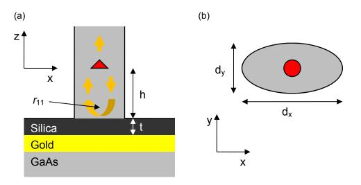
Fig. 2. (a) Bottom part of the elliptical nanowire geometry. (b) Cross-section.
