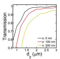
Fig. 10. Transmission  $\gamma$  to a 0.8 NA lens as function of semi-diameter  $d_{\gamma}$  for varying metal-contact overlaps o.
