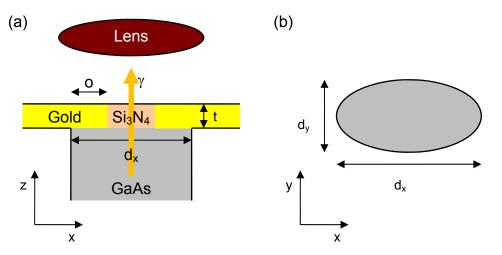
Fig. 7. (a) Top part of the elliptical nanowire geometry. (b) Cross-section of the GaAs nanowire.
