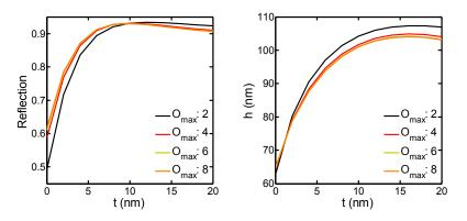
Fig. 4. Reflection and *h* as function of *t* and the number of included orders  $O_{max}$ . Parameters: Modes: 400 and  $R_{CD}$ : 3 µm. The number of required orders is studied in Fig. 4. We observe that convergence is obtained for approximately  $O_{max}$  = 6 included orders.
