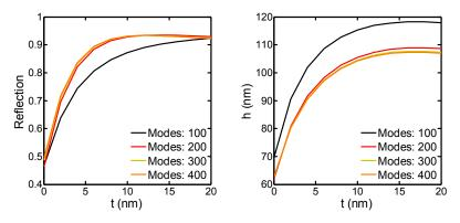
Fig. 3. Reflection (left) and ideal QD-mirror distance *h* (right) as function of the silica layer thickness *t* and the number of modes per order. Parameters: *O<sub>max</sub>*: 2 and *R<sub>CD</sub>*: 3 μm.
