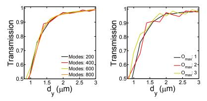
Fig. 8. Transmission  $\gamma$  to a 0.8 NA lens as function of semi-diameter  $d_y$  for varying number of modes (left) and for varying number of orders  $O_{max}$  (right).
