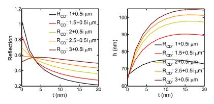
Fig. 6. Reflection and h as function of t and the radius R<sub>CD</sub> of the computational domain. Parameters: Modes: 400 and O<sub>max</sub>: 6
