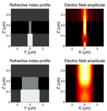
Fig. 11. Refractive index profile (left) of the top contact section shown in Fig. 2(a) for  $d_y = 0.8 \mu m$  (top) and  $d_y = 3 \mu m$  (bottom) for o = 200 nm. Corresponding electrical field amplitude profiles (right).
