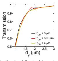
Fig. 9. Transmission  $\gamma$  to a 0.8 NA lens as function of semi-diameter  $d_y$  for varying radius R<sub>CD</sub> along the short semi-axis of the computational domain.
