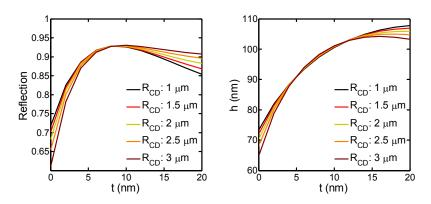
Fig. 5. Reflection and h as function of t and the radius R<sub>CD</sub> of the computational domain. Parameters: Modes: 400 and O<sub>max</sub>: 6
