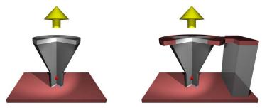
Fig. 1: Artistic illustrations of the elliptical photonic nanowire geometries. Optically pumped design (left) and electrically pumped design (right) implementing a top metal contact.
