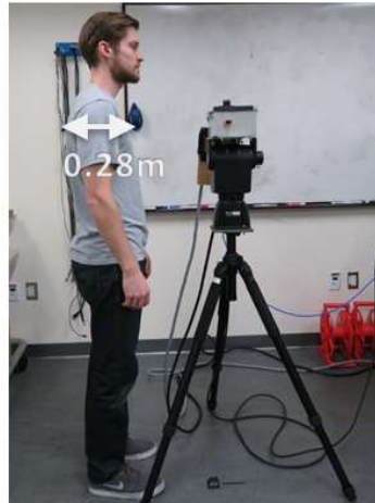
Fig. 3: Human blocker dimensions with the TX and RX. b_{\text{height}} = 1.8 m; b_{\text{breadth}} = 0.47 m; b_{\text{depth}} = 0.28 m; TX/RX height = 1.4 m.
