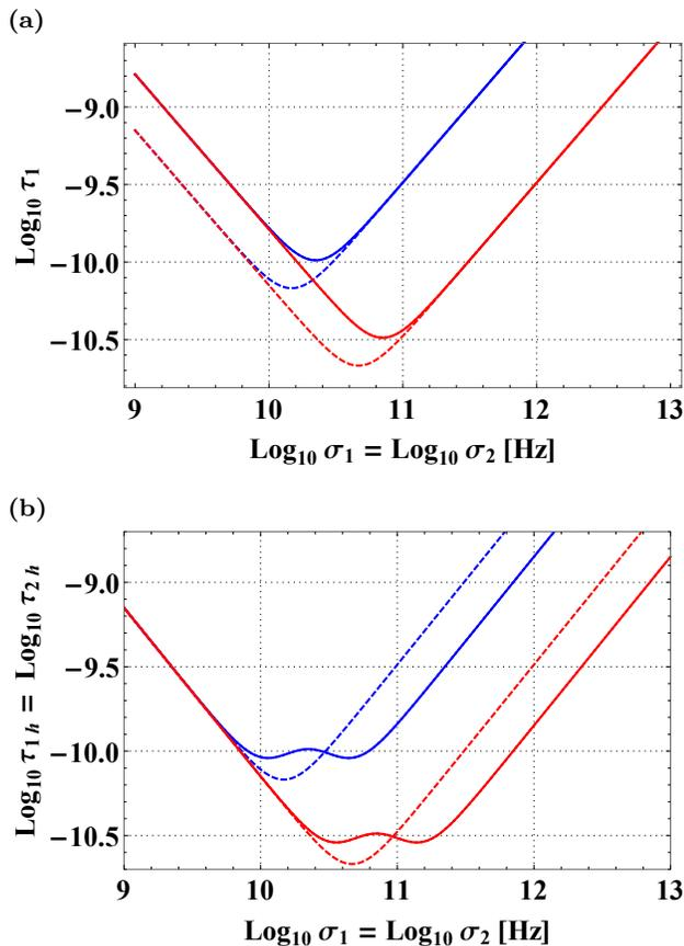
FIG. 6. Temporal widths a)  $\tau_1$  and b)  $\tau_{1h} = \tau_{2h}$ , given by the formulas (8) and (10) respectively, plotted as functions of spectral widths  $\sigma_1 = \sigma_2$  for the spectral correlation coefficient  $\rho = 0$  (dashed lines) and  $\rho = 0.9$  (solid lines) and for two different lengths of the standard SMF fibers connecting the source with Alice and Bob: 20 km (red lines) and 200 km (blue lines). All the plots were made for the detection timing jitter  $\tau_j = 0$ .
