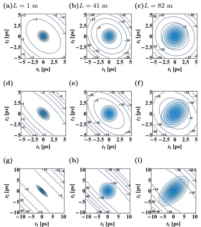
FIG. 8. The amplitude and phase of the biphoton wave function,  $\psi_L(t_1, t_2)$ . In the columns the propagation distances are: 1 m (a, d, g), 41 m (b, e, h) and 82 m (c, f, i). In the rows the initial spectral correlation is taken to be:  $\rho = 0.2$  (a, b, c),  $\rho = 0.5$  (d, e, f) and  $\rho = 0.9$  (g, h, i).
