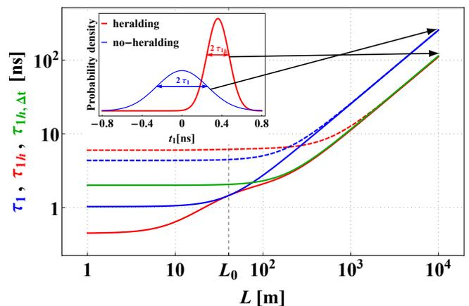
FIG. 3. The photon detection time widths  $\tau_1$  (blue),  $\tau_{1h}$  (red) and  $\tau_{1h, \Delta t}$  (green) as a function of the propagation distance  $L$  for  $\rho = 0.9$  and the detection timing jitter  $\tau_j = 0$  (solid lines) and  $\tau_j = 20$  ps (FWHM) (dashed lines). The inset shows the corresponding detection probability functions of finding a photon at time  $t_1$ .
