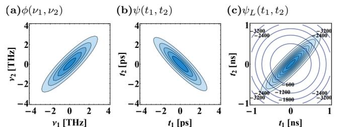
FIG. 1. The spectral (a) and temporal (b) wave functions  $\phi(\nu_1, \nu_2)$  and  $\psi(t_1, t_2)$  for  $L = 0$ . The functions are real-valued. (c) The phase and the amplitude of the photon pair state,  $\psi_L(t_1, t_2)$ , after a long propagation distance,  $L = 10$  km for the initial spectral correlation  $\rho = 0.9$ .
