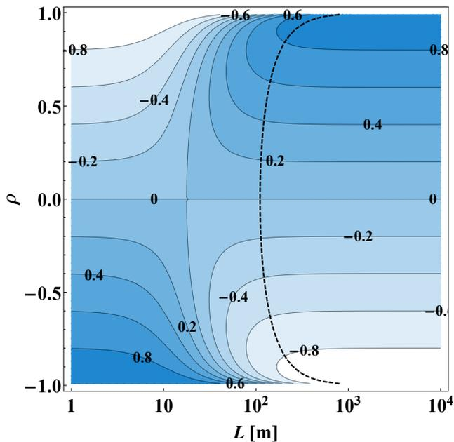
FIG. 2. The Pearson's correlation coefficient,  $r_{t_1 t_2}(L, \rho)$ , as a function of initial correlation  $\rho$  and SMF length  $L$ . The dashed contour indicates a distance,  $L_{0.95}$ , at which the correlation coefficient  $r_{t_1 t_2}(L, \rho) = 0.95\rho$ .
