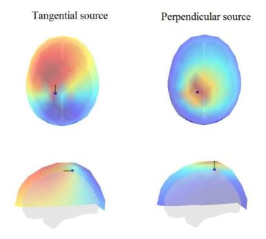
**Fig. 6** An instructive example of the effect of source orientation on the scalp electrodes. The sources are of unit strength and projected to the scalp. Top row and bottom row shows the locations (dot), orientation (arrow) of the sources (left: tangential source; right: perpendicular source) and corresponding topography in axial and sagittal view respectively
