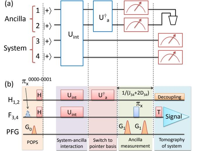
FIG. 4. (a) Quantum circuit to discriminate Lüders and von Neumann devices. (b) The NMR pulse-scheme to implement the circuit in (a).
