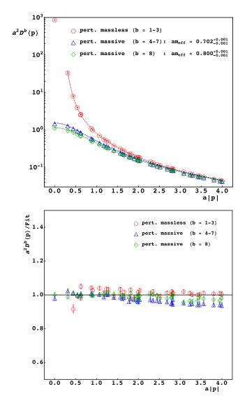
Figure 2. Top: Propagators in the unbroken SU(2) subgroup and the coset SU(3)/SU(2) for a  $V = 20^4$  lattice. The momenta are along the edges, and along all possible diagonals of the lattice, i.e.  $(p, 0, 0, 0), \ldots, (p, p, p, p)$ . Results are for the parameters  $\beta = 9.59055$ ,  $\kappa = 0.444462$ ,  $\lambda = 0.4118$ . The dashed lines denote the fits discussed in the text. Bottom: Differences of the lattice propagators and the fits.
