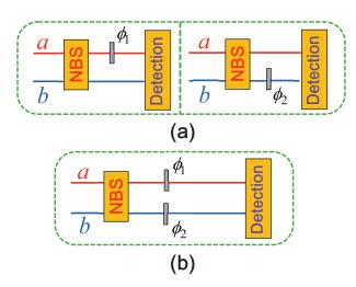
FIG. 2. Different phase delay ways of the interferometer: (a) Phase shift in the single arm is divided into single upper arm and single lower arm due to the intensities of the two arms are not equal. (b) Phase shifts in the two arms.
