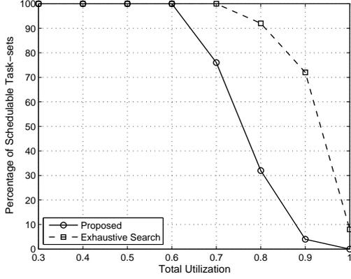
Fig. 1. Normalized percentage of the number of schedulable task-sets. The base-utilization of the real-time tasks are varied from  $[0.01+0.1 \cdot i, 0.1+0.1 \cdot i]$  where  $0 \leq i \leq 8, i \in \mathbb{Z}$ . The utilizations of the security tasks are generated from  $[0.11, 0.20]$ . For exhaustive search, we set  $P_{max} = 2500$  with search granularity  $\delta = 0.5$ .
