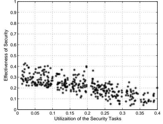
Fig. 3. The effectiveness of security is measured as  $\xi = \frac{\|\mathbf{T}^* - \mathbf{T}^{des}\|_2}{\|\mathbf{T}^{max} - \mathbf{T}^{des}\|_2}$ . The base-utilization of the real-time tasks are taken from  $[0.31, 0.4]$  and the base-utilization of the security tasks are varied from  $[0.01+0.1 \cdot i, 0.1+0.1 \cdot i]$  where  $0 \leq i \leq 3, i \in \mathbb{Z}$ . Hence the total utilization of the system varied from  $[0.3, 0.8]$ . Each utilization group contains 100 task-sets.
