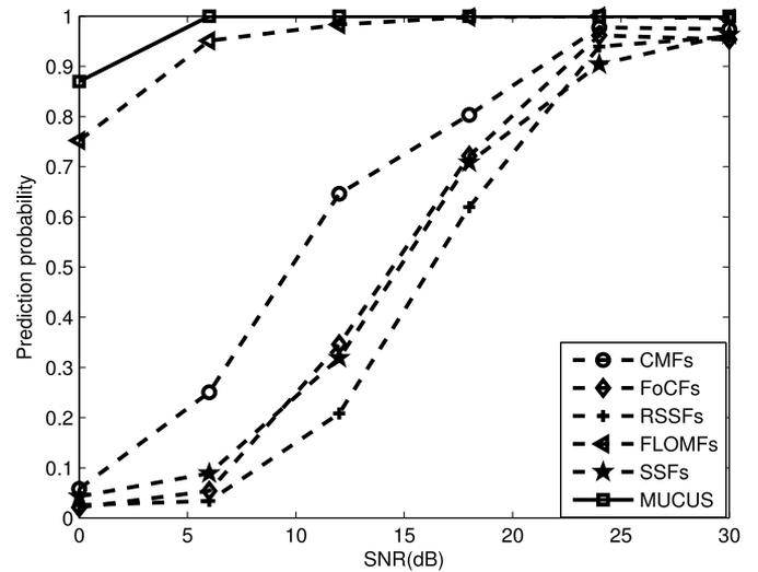
Fig. 6. The prediction performance of different algorithms versus different SNRs: impulse noise.
