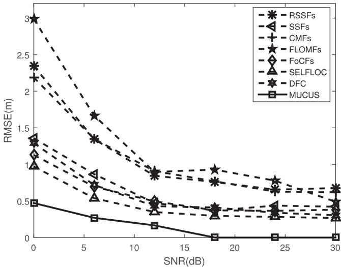
Fig. 5. The RMSE of different algorithms versus different SNRs: Gaussian noise.
