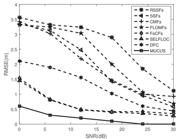
Fig. 7. The RMSE of different algorithms versus different SNRs: impulse noise.
