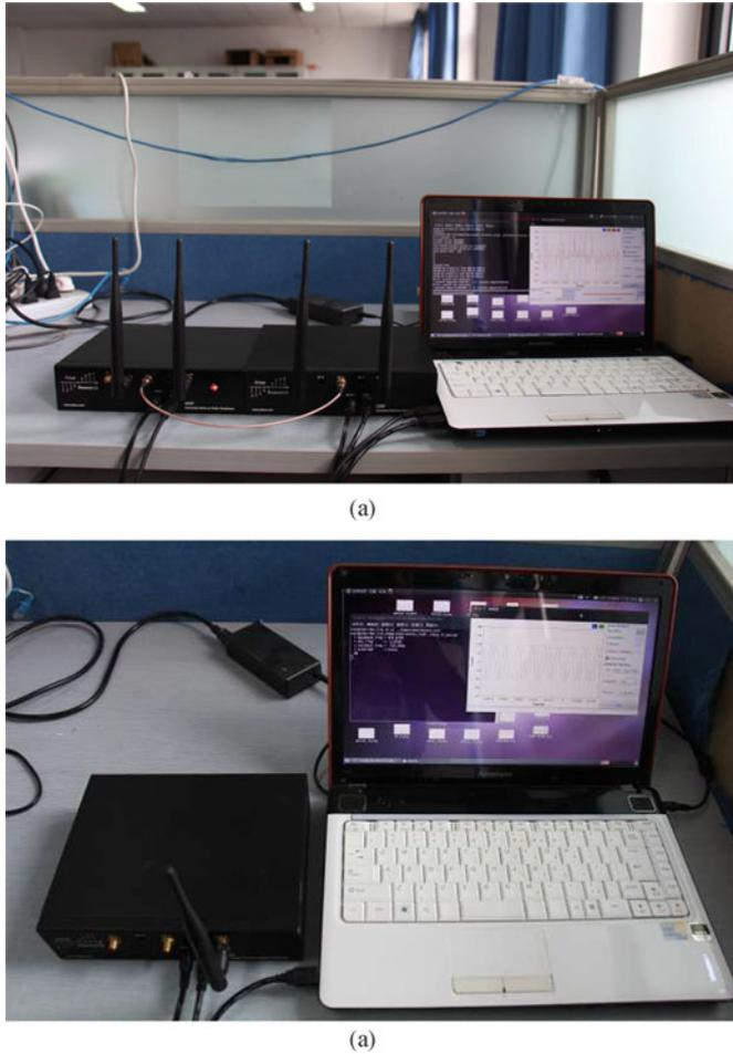
Fig. 8. The experimental testbed. (a) The USRP receiver platforms with 4 antennas. (b) The USRP transmitter platform with 1 antenna.
