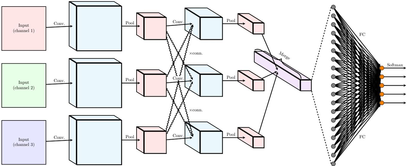
Fig. 1. Diagram of a simple cross-modal CNN for image classification, generated from a baseline CNN of the form  $[Conv \rightarrow Pool] \times 2 \rightarrow FC \rightarrow Softmax$ . Each of the three channels (RGB/YUV) of the input image receives its own CNN superlayer, with cross-connections inserted after the pooling operation, and full weight sharing in the fully connected layers. A more in-depth view of a potential cross-connection layout is provided by Figure 2.
