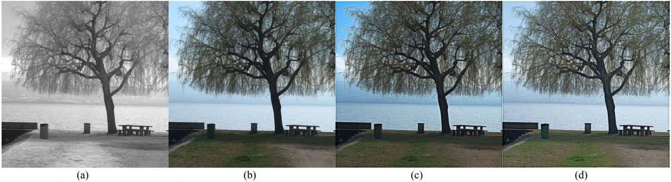
Figure 3. Near-infrared dehazing vs. coloring for ‘Lake’ image; (a) captured near-infrared gray image, (b) captured visible color image, (c) dehazed visible image with the proposed method, and (d) colored near-infrared gray image [12] (Please zoom in to the images to check details and colors).
