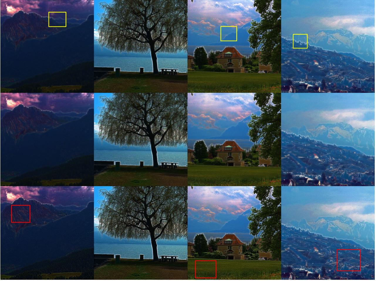
Figure 6. Experimental results for the used regularizations; (a) initial dehazed images via dark channel prior where alpha matting was not applied (first row), (b) dehazed images using gradient regularization (second row), and (c) dehazed images using gradient difference regularization (last row).
