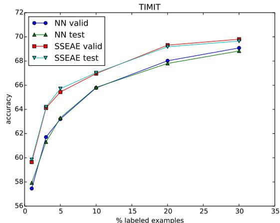
**Fig. 2.** Frame-based phoneme recognition accuracy (%) versus percentage of labelled training examples on the TIMIT database. NN: neural network trained with supervised back-propagation. SSSAE: our method. Both validation and test accuracy rates are shown. See Table 1 for the corresponding numerical values.
