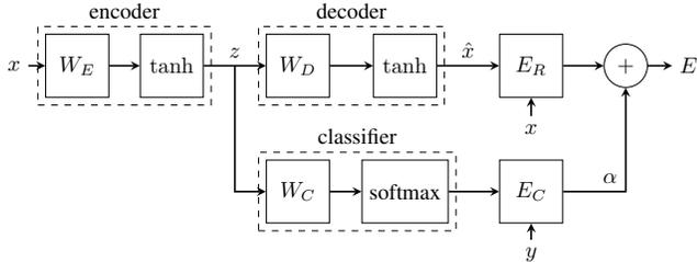
**Fig. 1.** Flow chart for the cost calculation in a single layer of the network. Three components are considered: encoder, decoder, and classifier. The loss is weighted sum of cross-entropy  $E_C$  and reconstruction loss  $E_R$ . If several layers are stacked together, only the encoder/decoder pairs are retained after training.
