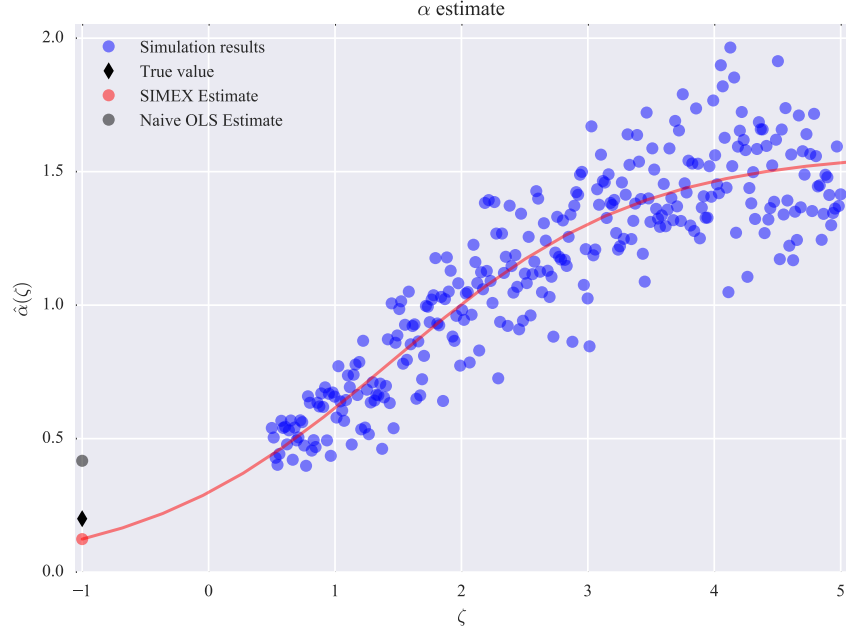
Figure 2: Illustration of the SIMEX procedure of Section 2.6. The error added to the measured data is indicated by the factor \zeta , with \zeta = -1 indicating the error-free state towards which simulation is extrapolated. This figure illustrates one realisation of the simulations for \alpha .
